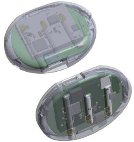
Second version of wearable node with an updated muscle fatigue tracking ASIC.
