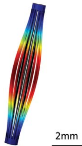
COMSOL Multiphysics simulation image of Nitinol as part of a catheter tip at a vibration mode
