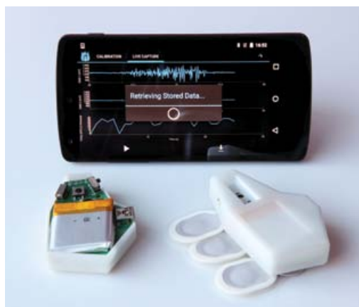
First version of wearable node with dedicated muscle fatigue tracking ASIC and custom Android monitoring application.
