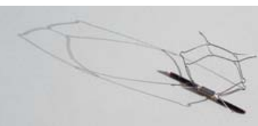
SAW pressure sensing implant for pulmonary artery
