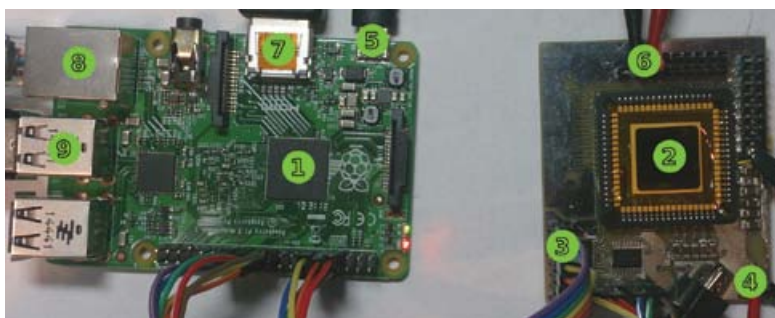
PCB evaluation platform of the neuron-processor interface prototype for developing on-chip classification methods for neural spiking activity (1) ARM core (2) NPI core (3) Serial I/O (4) Analogue power (5) Digital power (6) Sensor input (7) Display (*) LAN port (9) USB HDI
