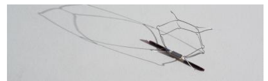
SAW pressure sensing implant for pulmonary artery.
