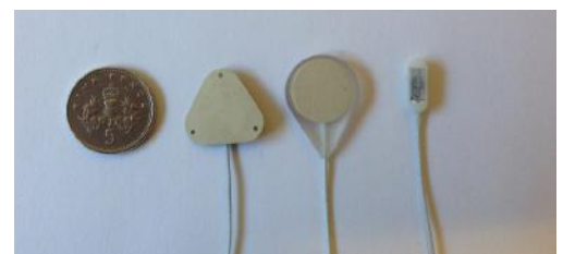
Antennas and sensor for Intracranial pressure monitoring.
