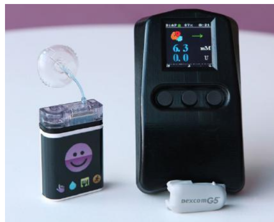
The Bio-inspired Artificial Pancreas (BiAP). Shown is the BiAP handheld unit which interfaces to a Dexcom G5 continuous glucose monitor and a Cellnovo Insulin Patch pump.
