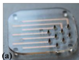
(a) Array of individually addressable microneedles which were coated with iridium oxide in order to sense pH changes. (b) Colour map of the pH distribution obtained with the microneedles device inserted into an ex-vivo perfused rat heart. Snapshots taken at the minutes indicated below each frame. The rat heart underwent two cycles of global heart ischemia/reperfusion. Ischemia occurred at t=8 min and 38 min while reperfusion at t=22 min and 52 min.
