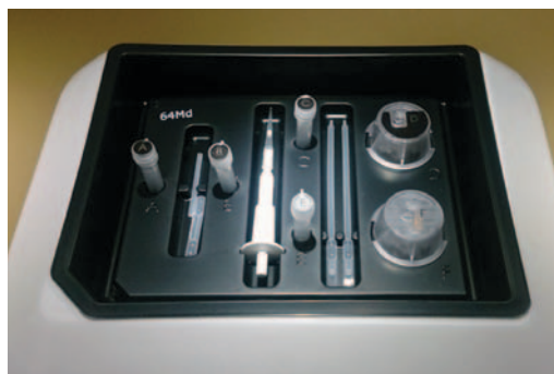
A prototype DNA test kit, incorporating a semi-conductor minilab, that allows live DNA testing
